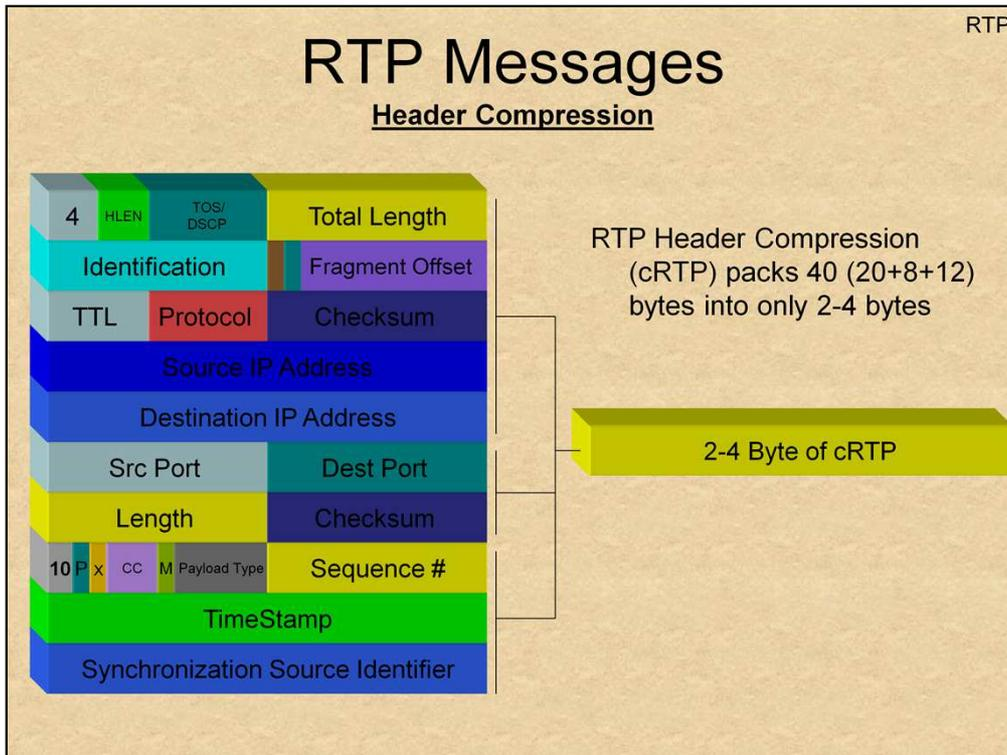
Even with a mere 12-bytes, RTP's header can be a concern. A dozen bytes may not seem like much, but along with IP (20 bytes) and UDP (8 bytes) – that's 40 bytes. In some cases, (e.g. G.729) this protocol header overhead is twice the payload. CRTP, the RTP header compression, enables to compress the header further – along with the UDP and IP headers – to a mere 2-4 byte value. This is feasible since many of the IP header fields are immutable, and certainly UDP ones are fully predictable.
