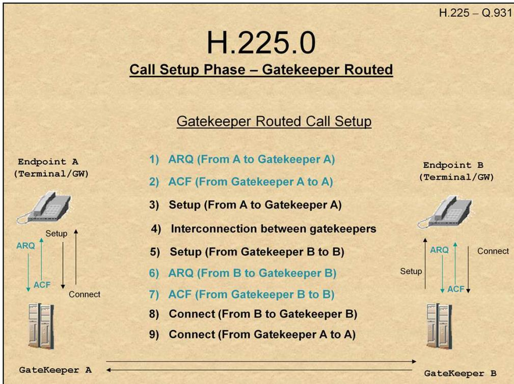
Gatekeeper routed configurations, as the name suggests, enable all calls to be routed through the gatekeepers themselves. Connection is not Point to Point, but Point-GateKeeper-GateKeeper-Point. This is useful to prevent cases wherein a rogue terminal can attempt connections without GateKeeper approval. In these configurations, the GateKeepers establish the call, and may configure FireWalls to enable specific connections, giving better control over VoIP calls.
