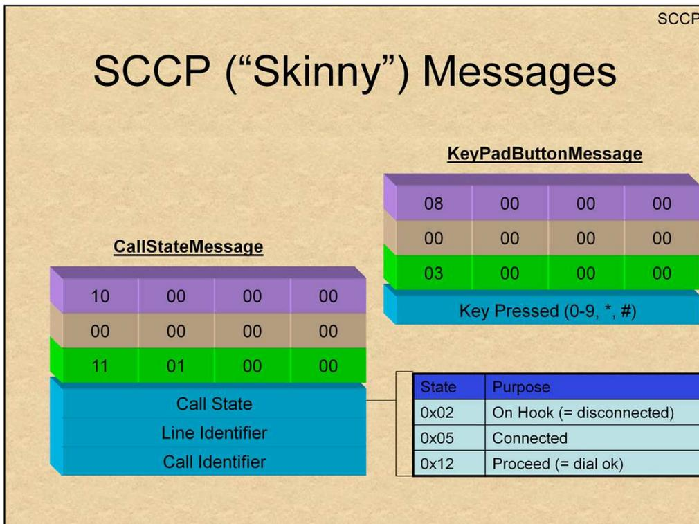
The slide above shows the important "dialing" messages that SCCP supports. These are the KeyPadButton Message (for each dialed digit) and the CallState Message. The latter is sent by the Call Manager to the Station at various stages of the call lifespan, with the codes specified in the table above.
