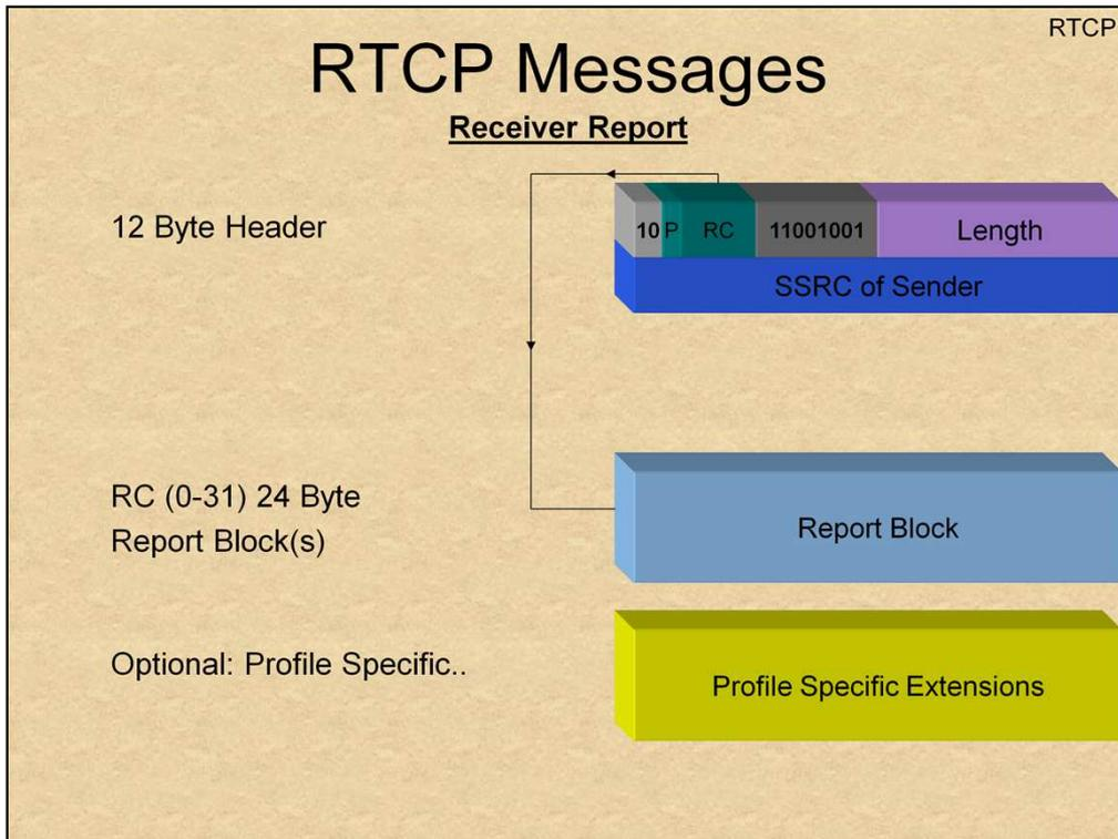
The Receiver Report (PT = 201) is identical to the Sender Report packet, with the exception that the Sender Info Block is omitted.
