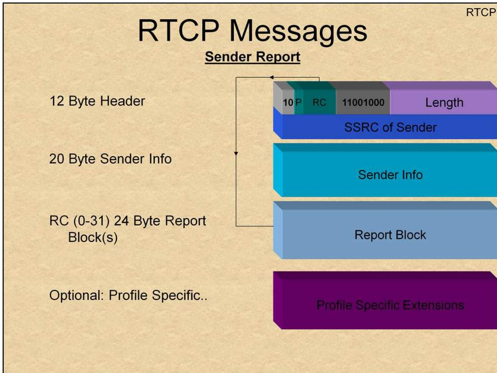
RTCP's "Sender Report" is comprised of a fixed 20-byte "Sender Info" block, and an optional 0-31 (5-bit value – RC) "Report Blocks". Each report block is 24 bytes.
