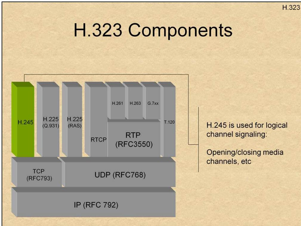
H.245 – “Control protocol for multimedia communication” defines the protocol that is used for logical channel control, or signaling. This involves setting up the transport channels for the various media streams.
