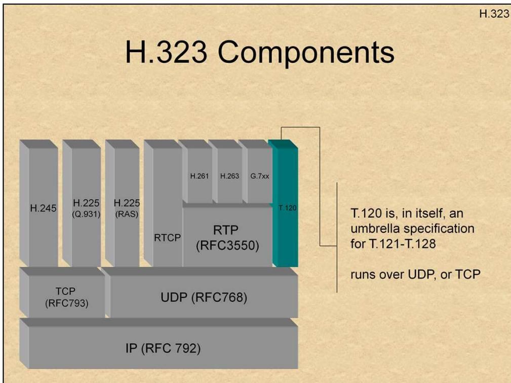
**T.120** is used for application data transfer over the H.323 framework. It is an umbrella specification for the following sub-protocols:
