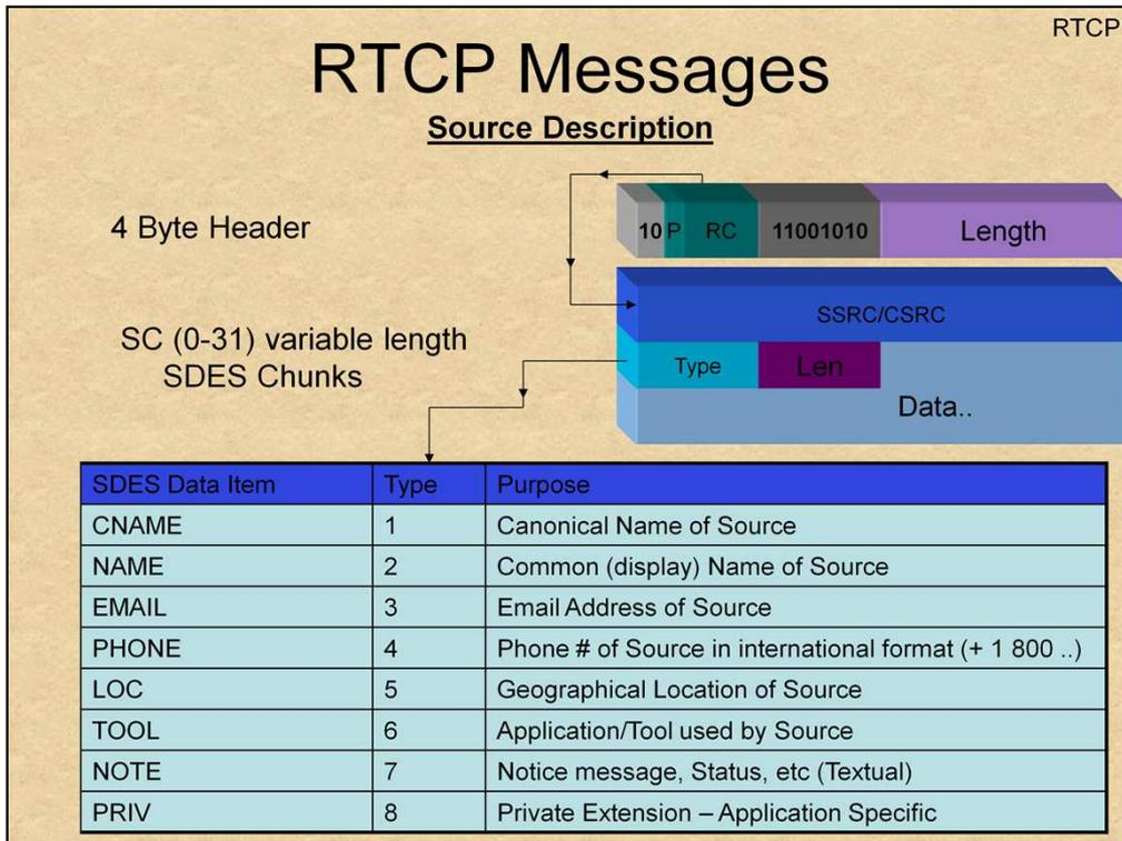
The Source Description (SDES) packets provide miscellaneous ancillary data about the source of the RTP stream. This is mostly for human purposes – providing the source's ID, phone #, location, etc. The table above summarizes the defined record types.
