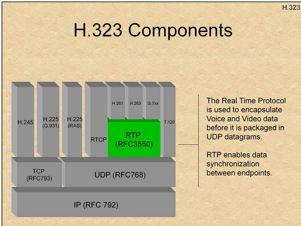
A key transport protocol used in H.323 is RTP – The Real Time Protocol (RFC3550). This protocol will be elaborated in greater detail in a few pages.
