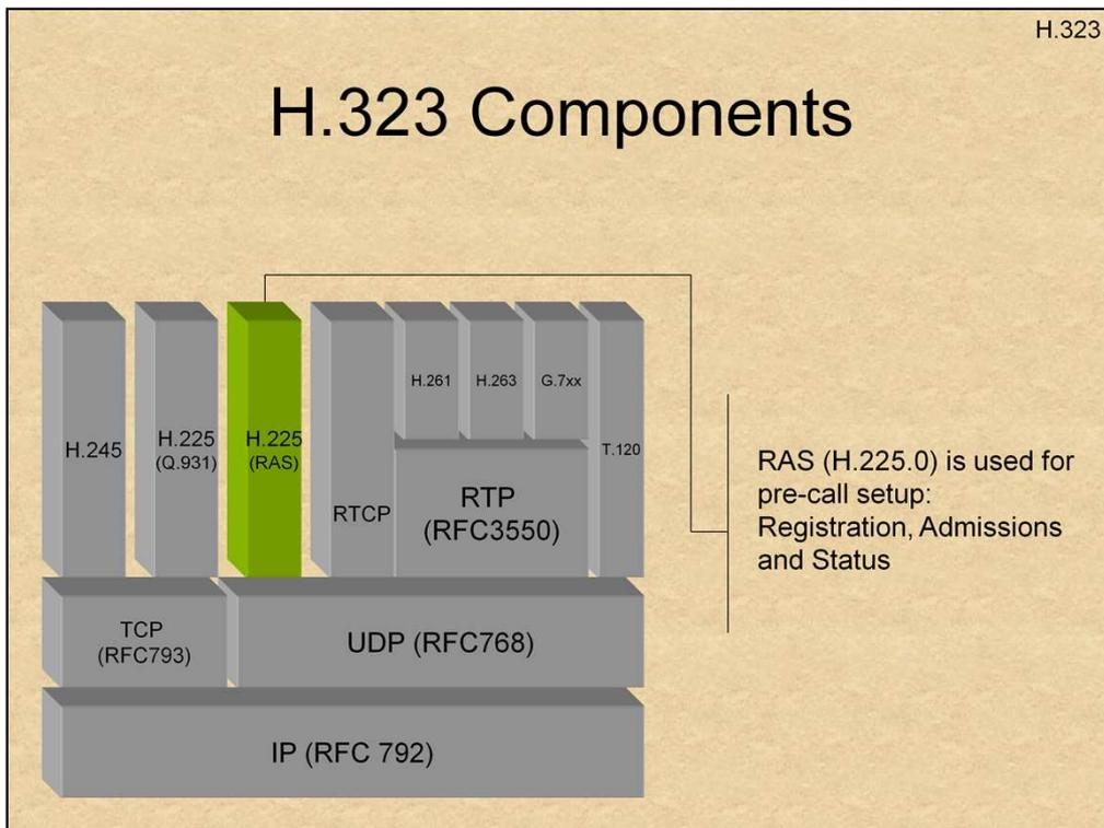
RAS is a sub-component of H.225 used for the pre-call setup stages, as well as modifying call parameters.
