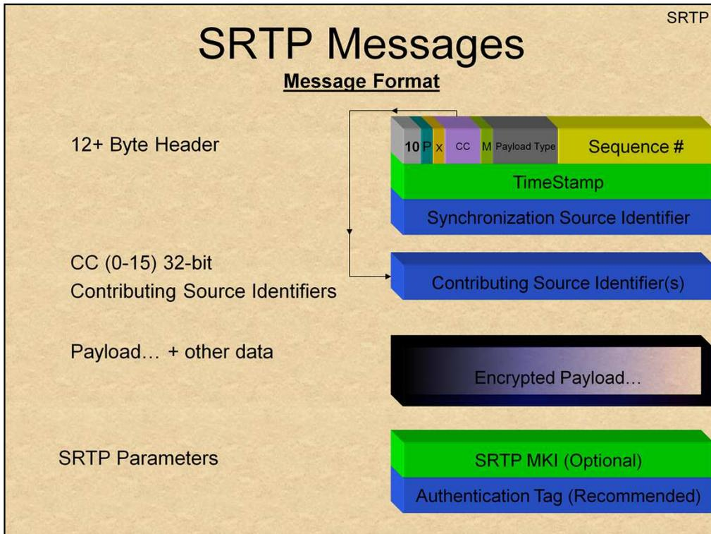
SRTP encrypts the RTP payload, and authenticates the entire packet. It piggybacks over normal RTP by appending two fields to an RTP message:
