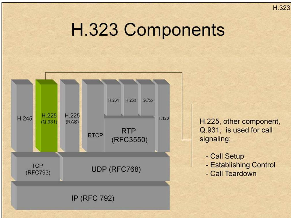
H.225.0 – “Call signalling protocols and media stream packetization for packet-based multimedia communication systems”
