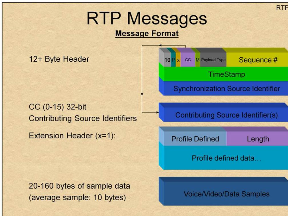
RTP Headers are fixed 12-byte headers, including only the necessary fields for transport management. The fields are listed below:
