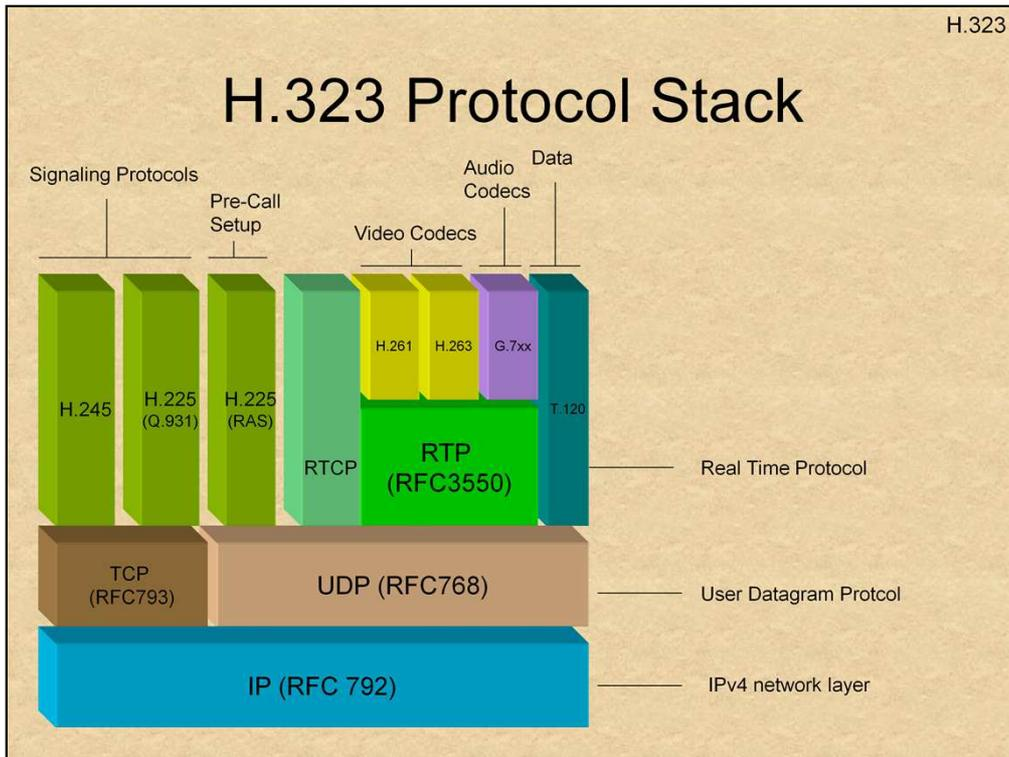
The above slide shows the H.323 “Protocol Stack” – and is an important illustration as to how all the various building blocks of H.323 “fit together”.
