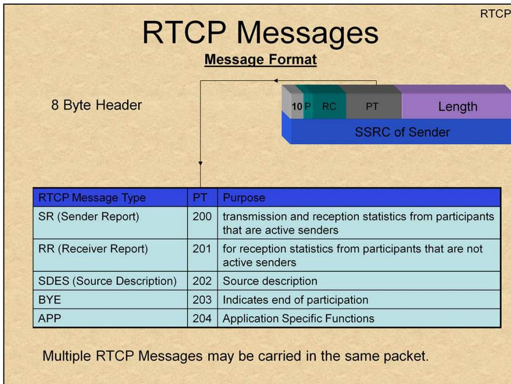
RTCP, The Real Time Control Protocol, works as a subset of RTP. It is meant to provide real time statistics, so as to enable QoS.
