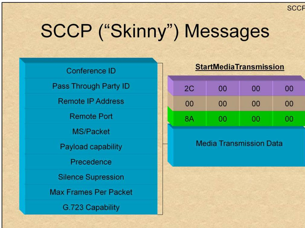
The "Start Media Transmission" is one of the more complex SCCP messages, due to its many fields. Its format is shown above, and in the following illustration.
