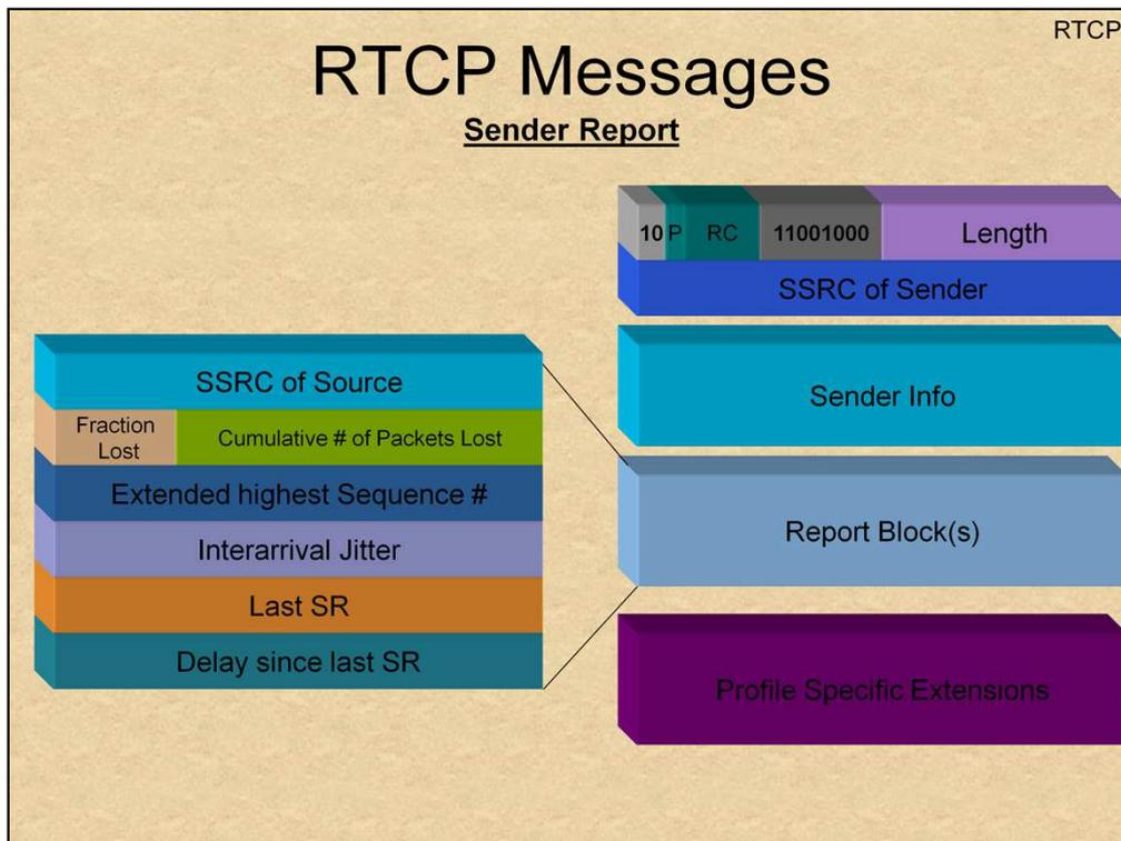
The “Report Blocks” provide more details as to the source, and allow the determination of network lag and round-trip time. Each is 24 bits, as follows:
